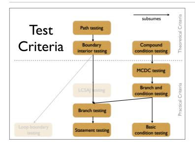
Boundary interior testing groups together paths that differ only in the subpath they follow when repeating the body of a loop. In other words, we follow each path in the CFG up to the first repeated node.
