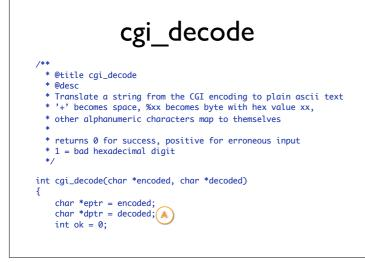
Here's an ongoing example. The function cgi\_decode translates a CGI-encoded string (i.e., from a Web form) to a plain ASCII string, reversing the encoding applied by the common gateway interface (CGI) on common Web servers. (from Pezze + Young, "Software Testing and Analysis", Chapter 12)
