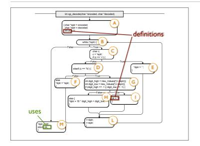
Data flow testing is based on the observation that computing the wrong value leads to a failure only when that value is subsequently used. A typical data flow testing criterion is therefore that the tests must exercise every pair (definition, uses) of a variable (such as "ok" in this example).
