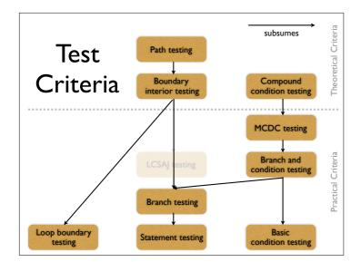
Another alternative is loop boundary testing which forces constraints on how loops are to be executed. This is a practical criterion.
