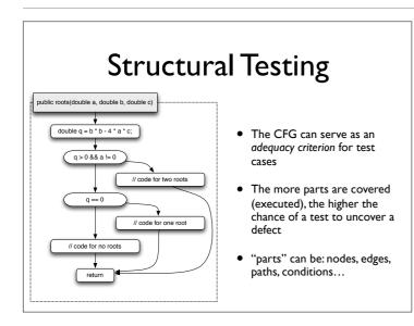
To talk about structure, we turn the program into a *control flow graph*, where statements are represented as nodes, and edges show the possible control flow between statements.
