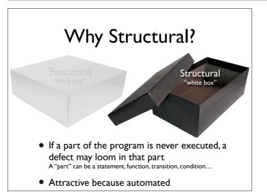
Structural tests are automated – and can be much more fine-grained than functional tests.
