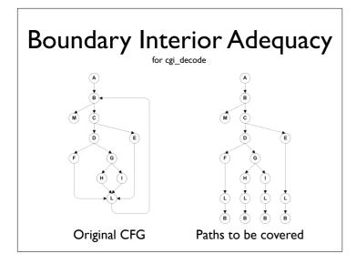
The graph at the right shows the paths that must be covered in the control flow graph at the left, using the "boundary interior" adequacy criiterion.
