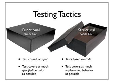
In contrast to *functional tests* (discussed the last time), *structural* tests are based on the code structure
