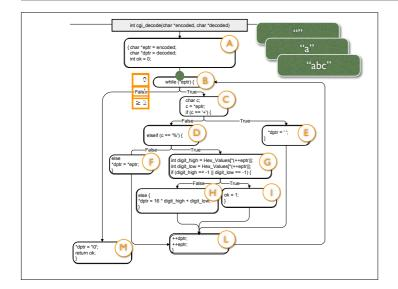
With these three test cases, we obtain loop boundary adequacy for the cgi\_decode main loop.
