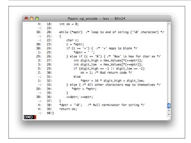
This is the output of the GCOV coverage tool for cgi\_decode. Each statement (each line) is annotated with the number of executions so far. Zero executions is suspicious and would be marked by "#####"; the tag "-" stands for lines without executable code.
